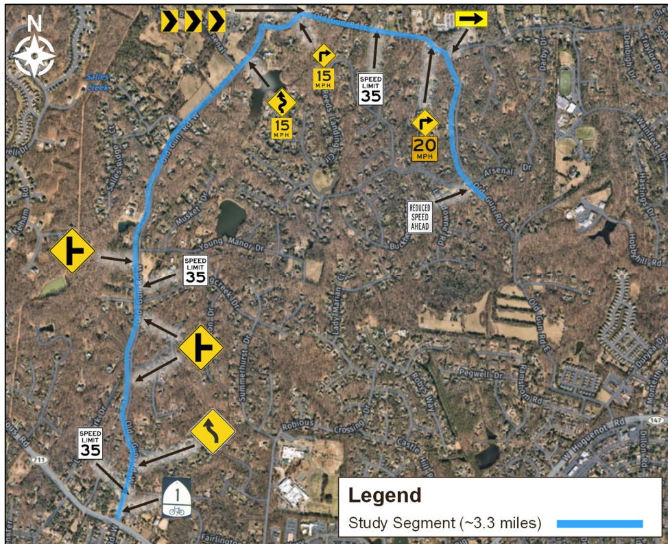
Figure 3: Existing Eastbound Signs
